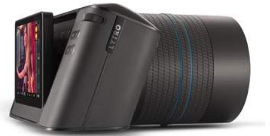
Lytro Illum plenoptic lightfield camera. The camera allows re-focussing after the photograph has been taken
